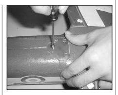
D. Mount main wing to fuselage using M4 x 10 screws.
