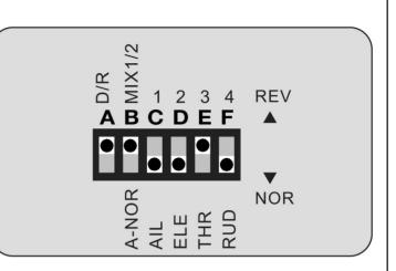
E. Channel 3 – Throttle reverse switch. The down position is normal mode and in the up position the function is reversed.
