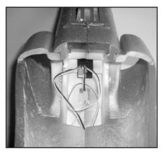
C. Insert the servo wire into the receiver matching the direction of the others.
