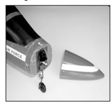
INSTALLING THE FRONT NOSE
