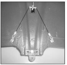
A. Install the aileron control rods, as shown in the picture.
