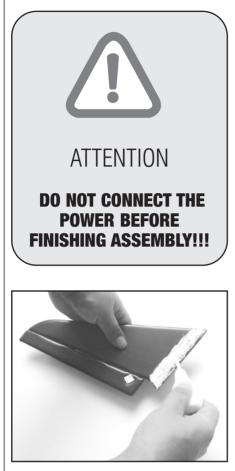
**INSTALL HORIZONTAL TAIL** Apply glue to inside edge of each tailplane half as per photo and mount to fuselage.
