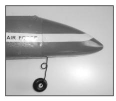
Line up the front nose with the white stripe so that it matches the fuselage line. Fix nose to fuselage with M2 x 4 screws.
