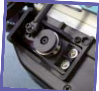
The high torque steering servo is inverted in the chassis, as you can see it has a built in servo saver
