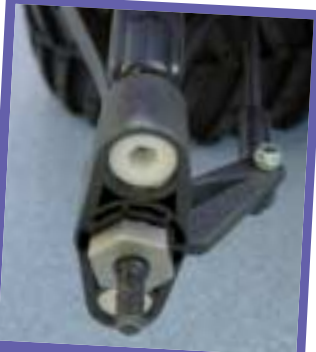
Delrin is used for the pivot ball adjuster nuts, see text. Alloy wheel hexes are often an upgrade on other Monster trucks
