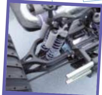
The top wishbone wraps around the shock bodies to protect them
