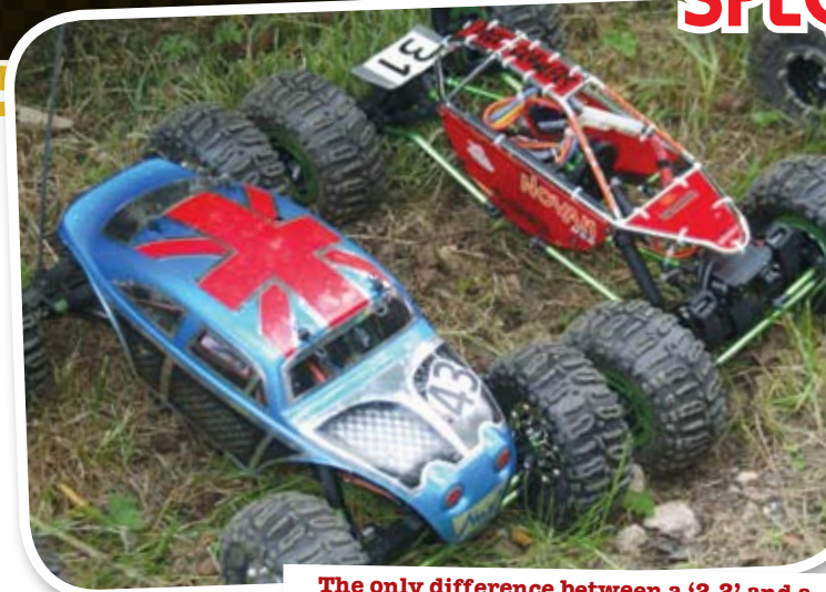
The only difference between a '2.2' and a 'Tuber' is a lexan shell or a tubular rollcage
