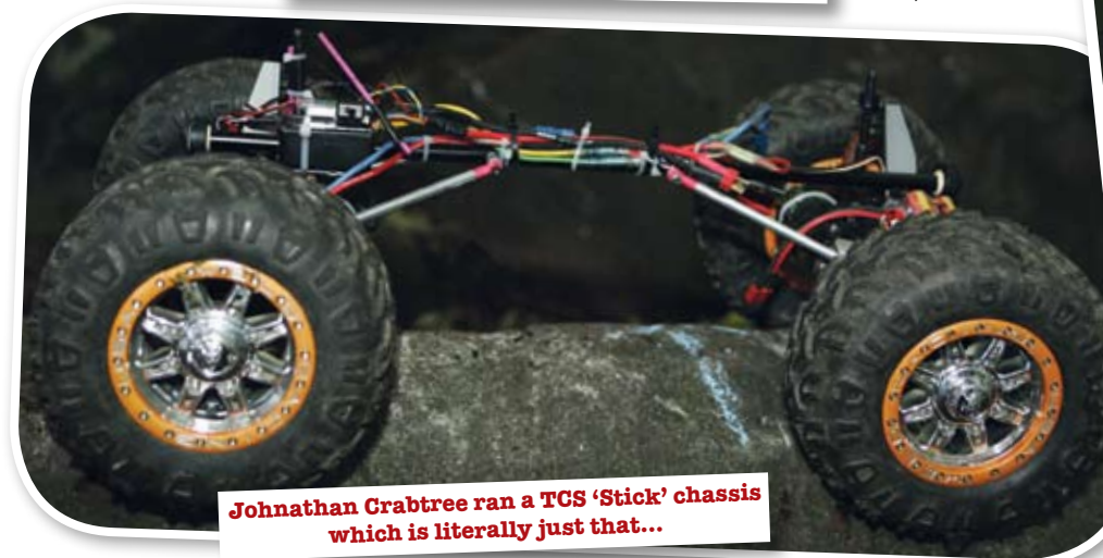
The only difference between a '2.2' and a 'Tuber' is a lexan shell or a tubular rollcage
