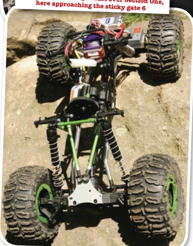
Mike Sager had a handful of lead shot in each of his Losi Rock Claw tyres, and no top plate on his unstoppable Axial
